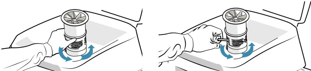
5. Remove the flow guide by lifting it.
