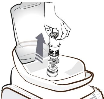
6. Put on a pair of gloves and pull the propeller, holding it firmly to take it out. Remove all debris (leaves, stones, etc.) which may be blocking the propeller.
